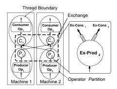
Figure 6: Exchange Architecture
