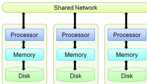
**Figure 2.1:** Shared-nothing architecture for parallel processing.
