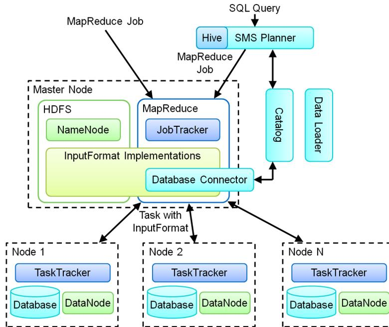
**Figure 4.4:** Architecture of the HadoopDB system, which has a hybrid design that combines MapReduce systems and centralized databases.
