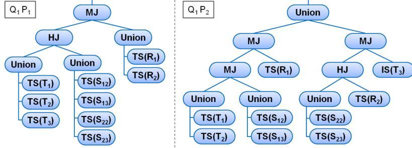
**Figure 2.4:**  $Q_1P_1$  and  $Q_1P_2$  are plans that can be generated by optimizers in parallel database systems for our example query  $Q_1$ . IS and TS are respectively index and table scan operators. HJ and MJ are respectively parallel join operators based on hash and merge. Union is a bag union operator.
