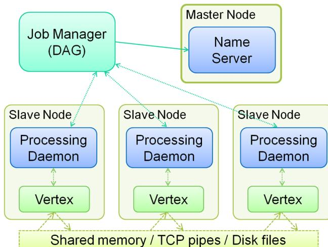
Figure 5.2: Dryad system architecture.
