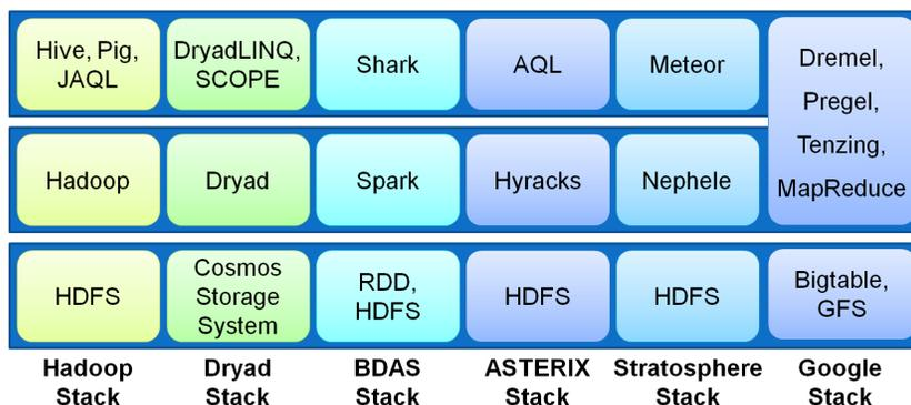
**Figure 5.1:** Typical dataflow software stacks along with the Hadoop stack.
