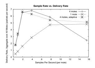
Fig. 15. Per-mote sample rate versus aggregate delivery rate.
