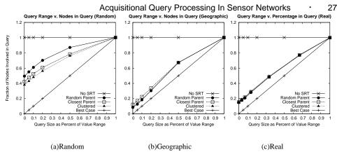
Fig. 9. Number of nodes participating in range queries of different sizes for different parent selection policies in a semantic routing tree (20x20 grid, 400 nodes, each point average of 500 queries of the appropriate size.) The three graphs represent three different sensor-value distributions; see the text for a description of each of these distribution types.
