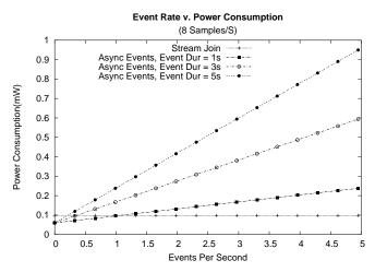
Fig. 7. The cost of processing event-based queries as asynchronous events versus joins.
