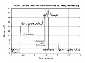
Fig. 3. Phases of Power Consumption In TinyDB ACM Transactions on Database Systems, Vol. V, No. N, Month 20YY.
